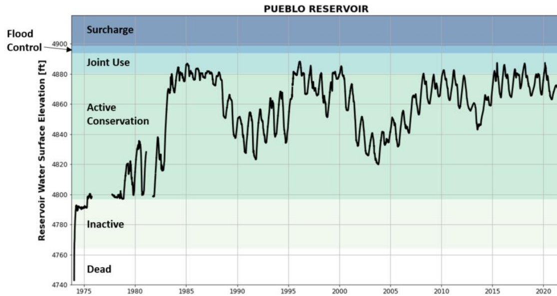
Figure 2-2: Historical Pueblo Reservoir Water Surface Elevation timeseries.
